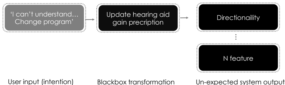
Figure 6.3: Two examples of mental models. The upper illustration shows a match between user intentions and the system output with regard to volume changes. The lower illustration shows a mismatch between the user intentions and the system output for hearing aid program change.
