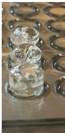
Figure S1 PU surface modified with NIPAAm showing gelation at high monomer feed concentration.
