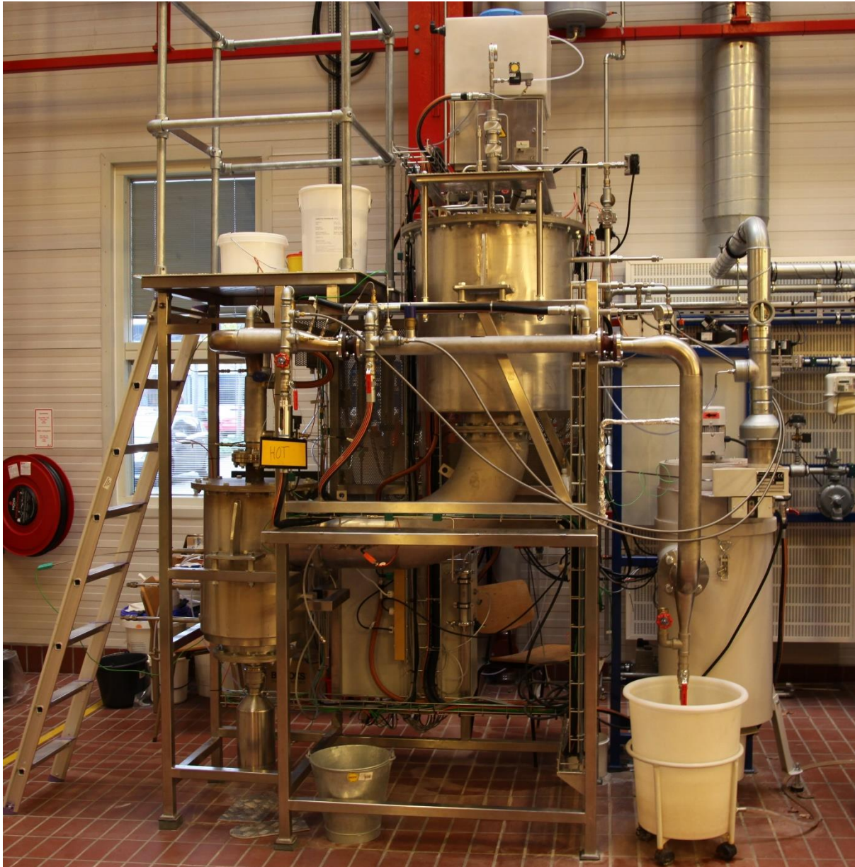
Figure 3.2: Picture of the pilot scale cyclone reactor setup
