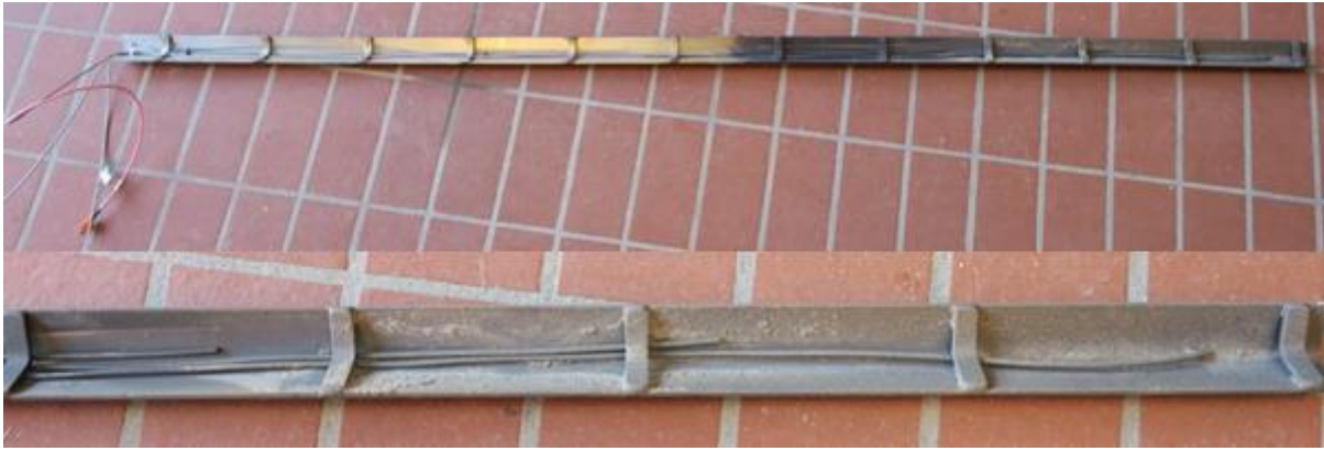
Figure 5.12: Pictures of assembled thermocouple array
