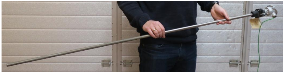
Figure 5.13: Picture of large k-type thermocouple for industrial use
