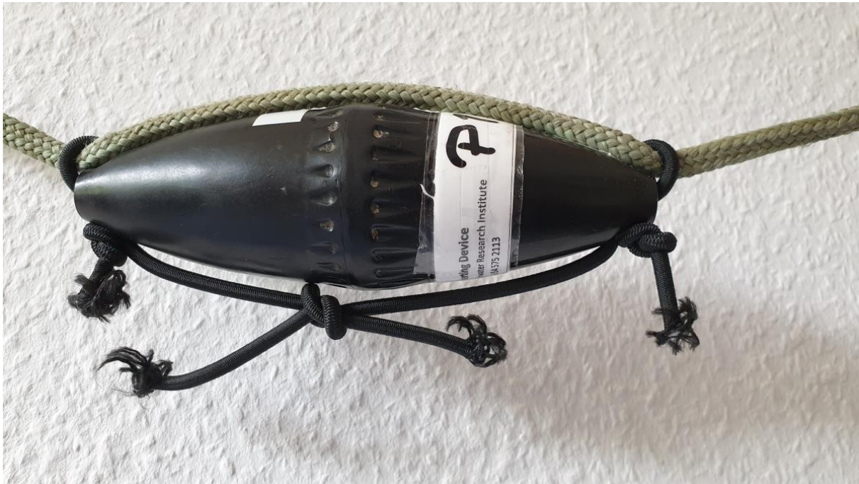
Figure 3: A PAL.v2 attached to a gillnet bridle. The PAL was marked on the battery compartment (right) to ensure fishers positioned them all pointing in the same direction.
