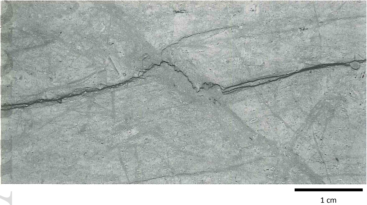
Fig. 6. Stylolite following compaction bands (photo: Ida Lind, Tidsskriftet Varv 1993, 2, front page).
