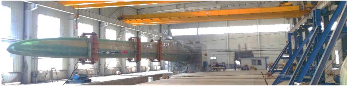
Figure 5. Setup of a full-scale blade test under combined flapwise bending and torsion [28]. The desired state of combined bending and torsion is achieved by shifting the loading lines (force action lines) in such a way that they do not pass the shear centers of blade sections. The step-wise static load is applied to collapse the blade.
