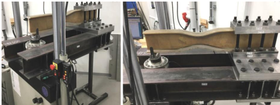
Figure 7. A tapered beam with adhesive joint interfaces [48]. The adhesive failure initiates in the gauge area remote from boundary conditions and load application points.
