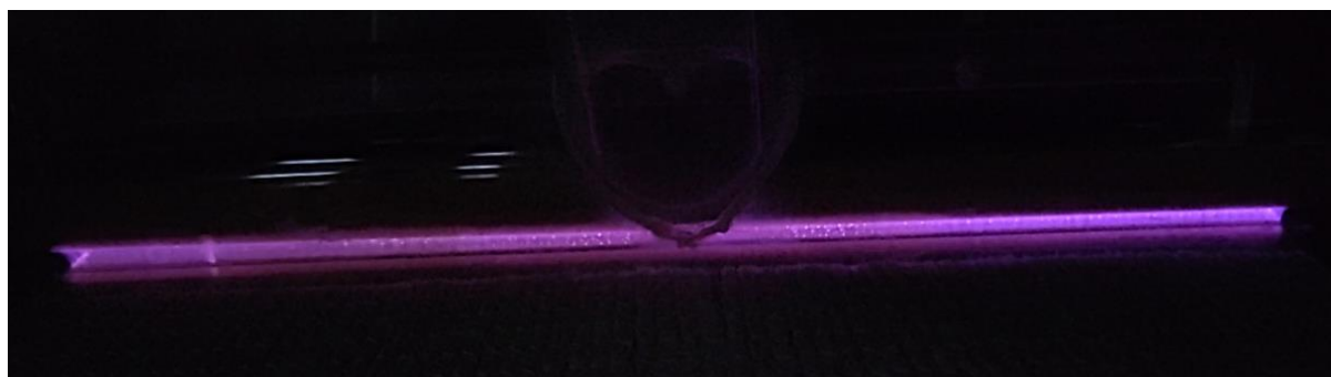
Fig. 2. A photo of the DBD in He/OFB gas mixture (gap: 2.0 mm, MR value: 0.45 %). The purple colour indicates photo-emission from the DBD between the cylindrical powered electrode and the ground electrode.
