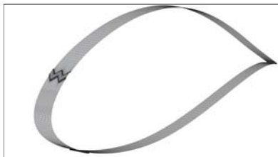
Figure 6. Perspective view of ZZ on airfoil. The entire span wise domain is shown
