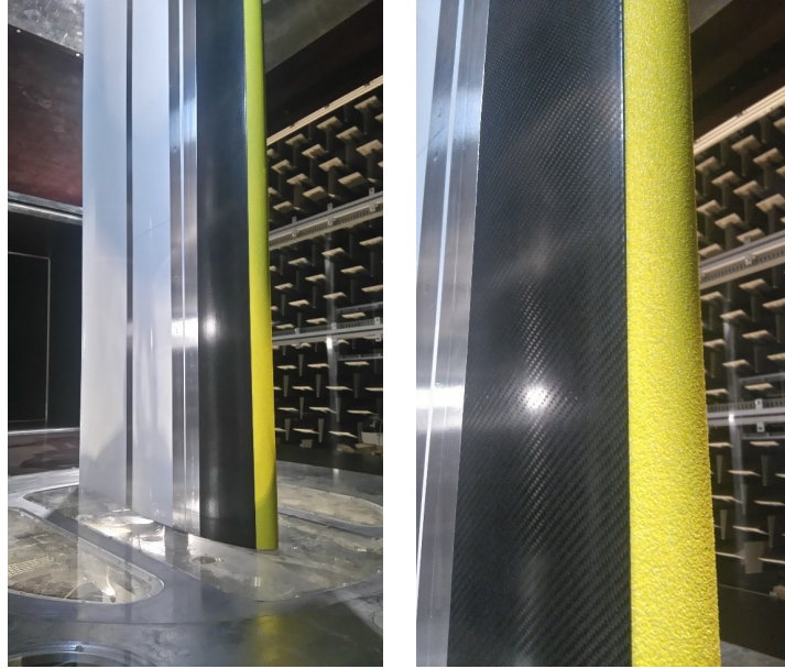
Figure 4. The NACA 63 3 -418 airfoil in the PLCT test section with the LE that includes a cavity, but no pressure taps. Left: The airfoil mounted with SP P40 at LE in the bottom of the cavity. Right: A close-up of the same configuration.
