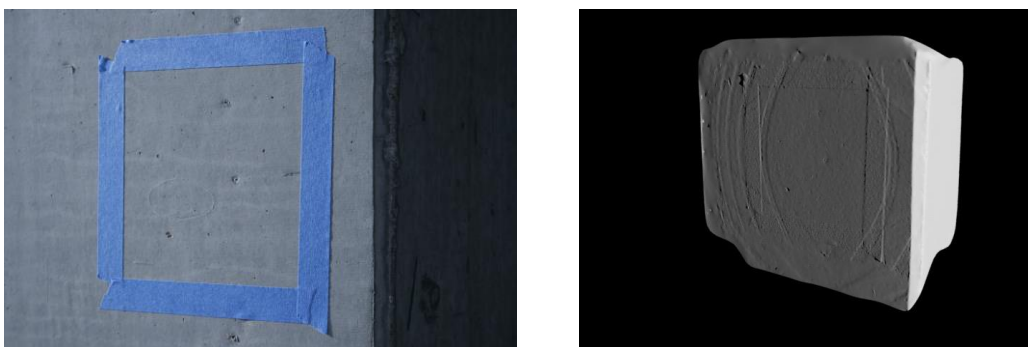
Figure 1. The left side is one of a small number of images acquired of a concrete pillar with masking tape. The right side is an initial 3D surface reconstruction showing surface structure and masking tape. The semi-circular surface features are artefacts due to insufficient image overlap.
