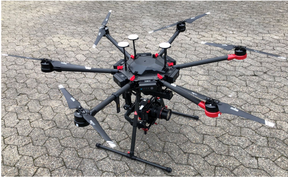
Figure 3.6: The DJI Matrice 600 Pro used in the project, equipped with the Canon EOS DS5 and the Ronin gimbal.
