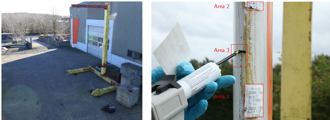
Figure 3.8: Left: Mock-up for testing purposes of drone autopilot and SfM. Right: Close-up of the blade tip leading edge with three areas selected for replication and validation in the laboratory.
