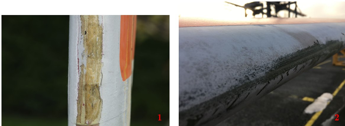
Figure 2.4: 1) Example of delamination on test specimen. 2) Example of both erosion and delamination on a 3 year old blade decommissioned due to structural manufacturing defects.
