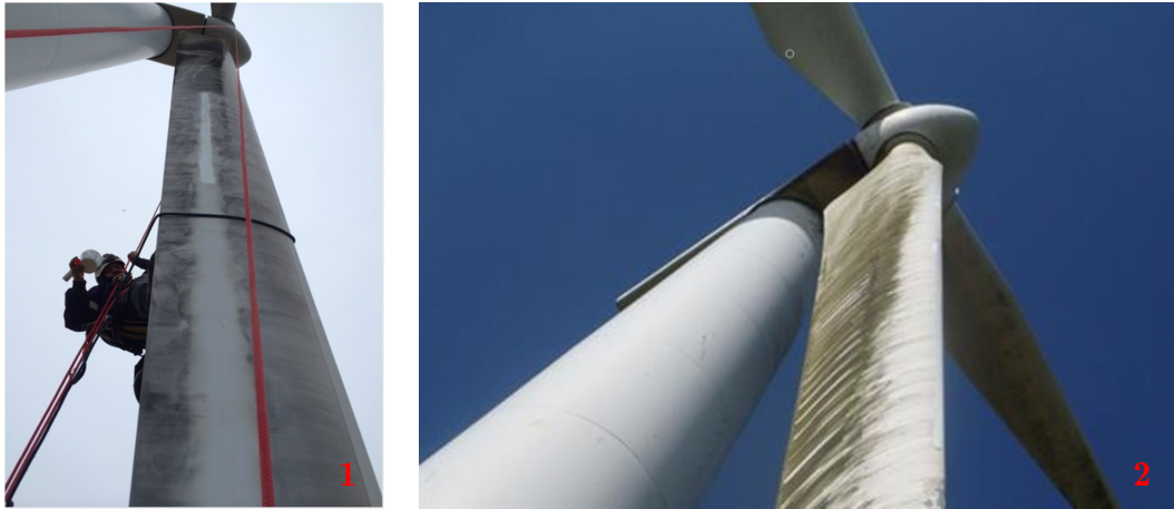
Figure 2.2: 1) Example of a blade with dirt and bugs. 2) Example of blade with moss and dirt from [9].
