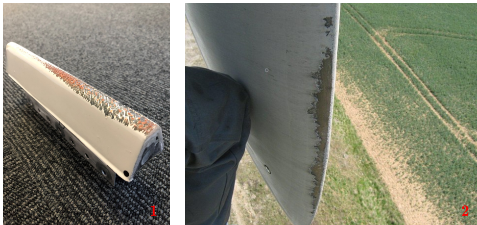
Figure 2.3: 1) Example of erosion from a rain erosion test. 2) Example of delamination on blade tip from [10].
