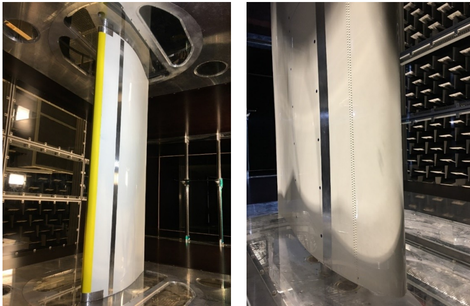
Figure 3. The NACA 63 3 -418 airfoil in the PLCT test section. Left: The airfoil mounted with SP P40 at LE. Right: The airfoil mounted with ZZ of height 0.4 mm at 10% c at PS and 2% c at SS.
