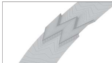
Figure 7. Closeup of ZZ tape grid. The entire span wise domain is shown
