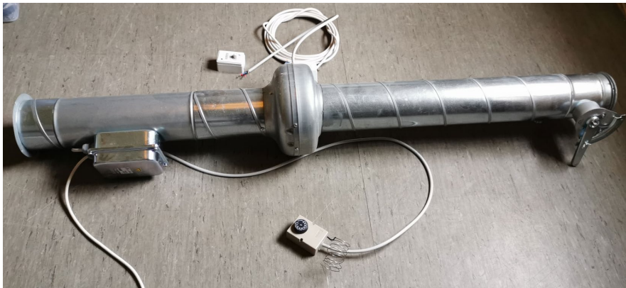
Fig. 5.6: Pre-assembled air conditioning rig - manual air flow control valve (right), adjustable fan with (middle), heating register with variable power (left).
