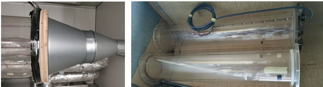
Fig. 5.7: Example for integration of an transparent Plexiglas-pipe with three junctions - currently used in another project (left); two plexiglas pipes with flanges on stock - 1500 x 240 mm, (right).
