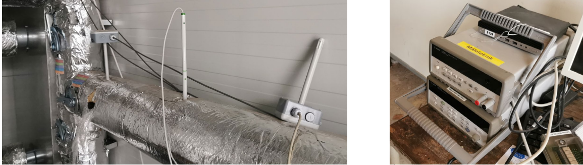
Fig. 5.5: Two combined humidity and temperature sensors and one anemometer for air property measurements (left); Agilent data logging equipment with analogue data logging cards (right).
