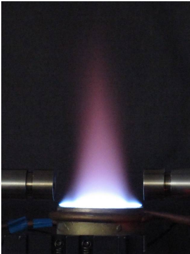
Figure C2: Visible picture of the methane/air flame at \phi = 1 . Lens adapters are also seen.
