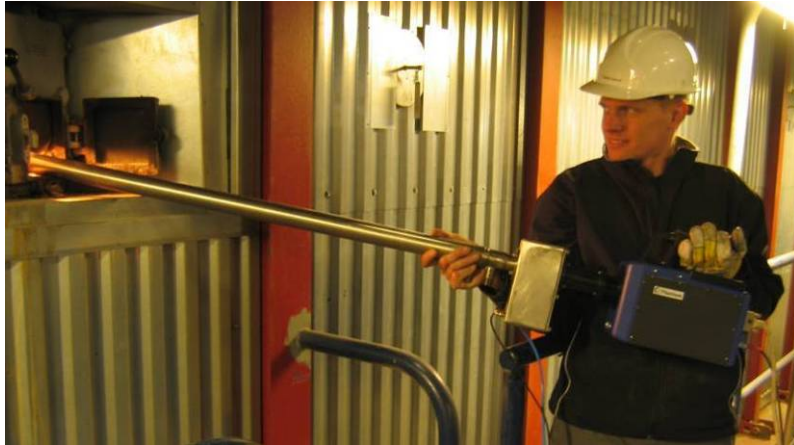
Figure 23 Inspection of flame using IR-camera with water-cooled endoscope optics.
