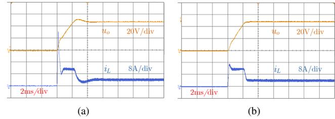
Fig. 12. Experimental results of system start-up response ( $u_o : 0 \text{ V} \rightarrow 48 \text{ V}$  with CPL power 192 W). (a) Cascaded PI control. (b) Proposed controller.
