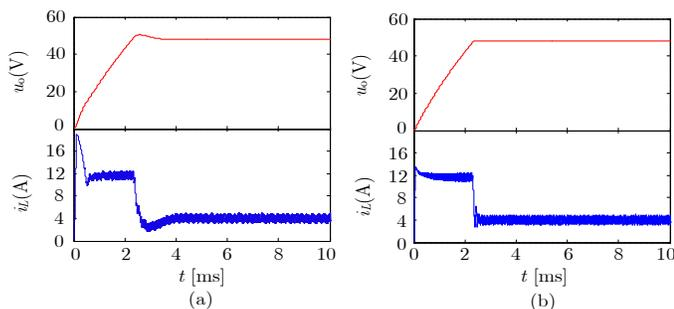
Fig. 6. Simulation comparison of system start-up response. (a) Cascaded PI controller. (b) Proposed controller.
