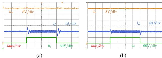
Fig. 15. Experimental results of system performance with a source-bus voltage step change. (a) Cascaded PI control. (b) Proposed controller.
