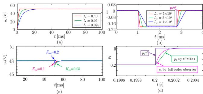
Fig. 5. Simulated dynamic response of load-bus voltage and disturbance estimation with different control parameters. (a) Load-bus voltage start-up response with different  $\lambda$ . (b)  $S^2MDO$  dynamic convergent response with different  $L_c$ . (c) Load-bus voltage dynamic response with different  $K_{sw}$ . (d) Comparison of disturbance-estimation dynamics using  $S^2MDO$  and conventional full-order disturbance observer.
