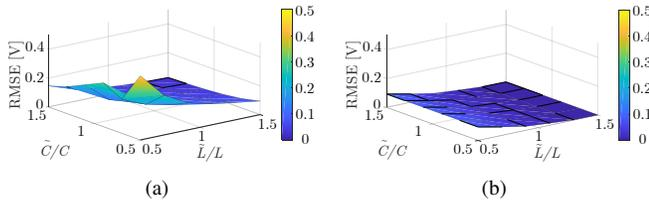
Fig. 10. Simulation comparison of load-bus voltage tracking RMSE with model uncertainties. (a) Cascaded PI controller. (b) Proposed controller.
