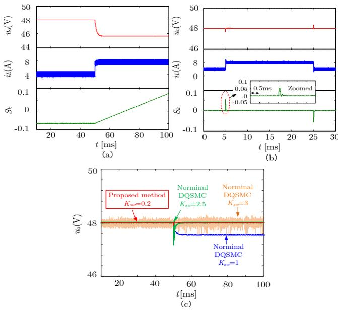
Fig. 9. Simulation comparison of sliding function dynamics and chattering with CPL disturbances. (a) Sliding-function dynamics using nominal DQSMC. (b) Sliding-function dynamics using proposed controller. (c) Chattering suppression comparison between nominal DQSMC and proposed controller.
