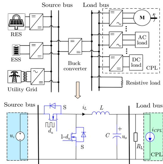
Fig. 1. Topology of a DC-DC buck converter feeding CPLs in a dc MG.
