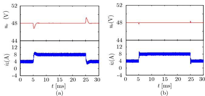
Fig. 7. Simulation comparison of system dynamic response with step CPL disturbances. (a) Cascaded PI controller. (b) Proposed controller.
