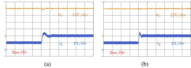
Fig. 13. Experimental results of system dynamic response with a CPL power injection (192 W  $\rightarrow$  384 W). (a) Cascaded PI control. (b) Proposed controller.
