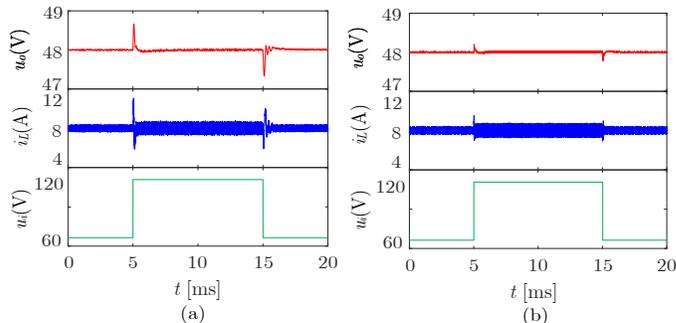
Fig. 8. Simulation comparison of system dynamic response with source-bus voltage disturbances. (a) Cascaded PI controller. (b) Proposed controller.
