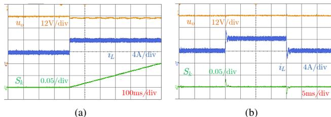
Fig. 16. Experimental results of system and sliding function response with a CPL step change. (a) Nominal DQSMC. (b) Proposed controller.
