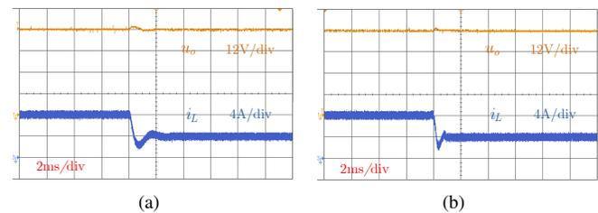
Fig. 14. Experimental results of system dynamic response with a CPL power remove (384 W  $\rightarrow$  192 W). (a) Cascaded PI control. (b) Proposed controller.
