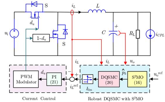
Fig. 3. Block diagram of the proposed composite robust DQSMC scheme in a multi-loop framework.
