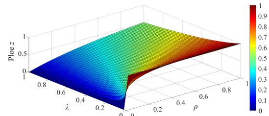
Fig. 4. Relationship between parameters  $\rho$ ,  $\lambda$  and closed-loop pole  $z$ .
