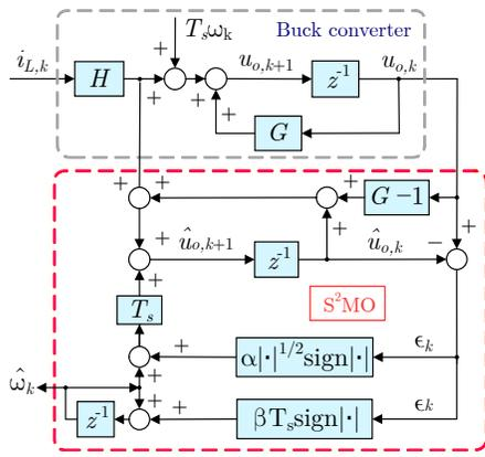
Fig. 2. Block diagram of S<sup>2</sup>MDO for lumped disturbance estimation of a buck converter.
