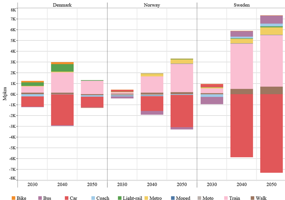
Fig. 6. Modal shift in inland passenger transport in the Scandinavian countries obtained with TIMES-NordicEMS in the Base scenario.
