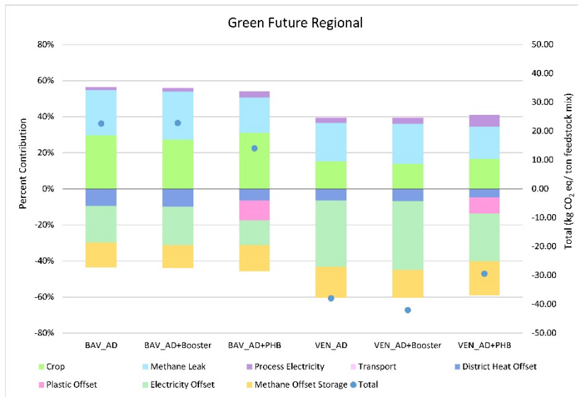
Figure 2-4 Global warming potential for a future with a theoretical green energy mix. Scenarios are named by the first three letters of the region (VEN or BAV) followed by each technology scenario (AD, AD+Booster, AD+PHB). Source: (G. Croxatto Vega et al., 2020).
