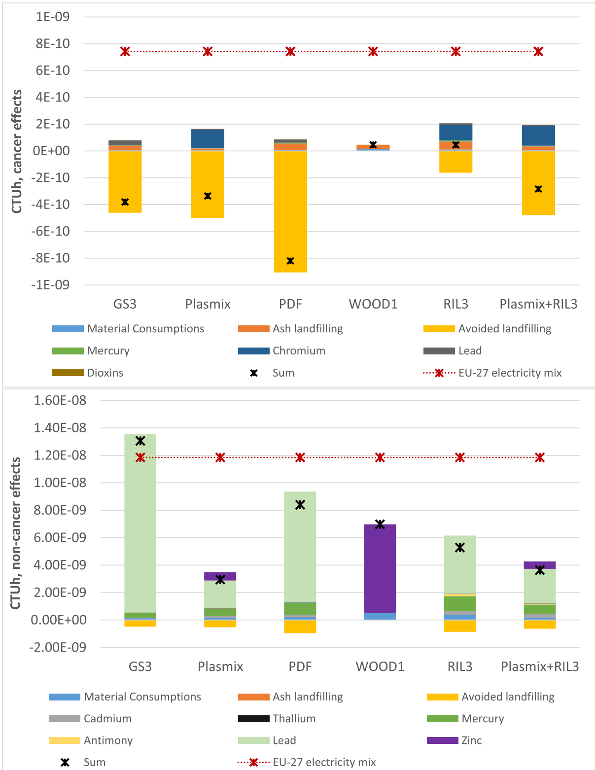
Fig. 10. LCIA results for the gasification of some of the analysed wastes, with reference to the “Human toxicity, cancer effects” (up) and “Human toxicity, non-cancer effects” (bottom) impact categories. Data have been compared with those associated to the European electricity mix. CTUh = Comparative Toxic Unit for humans.
