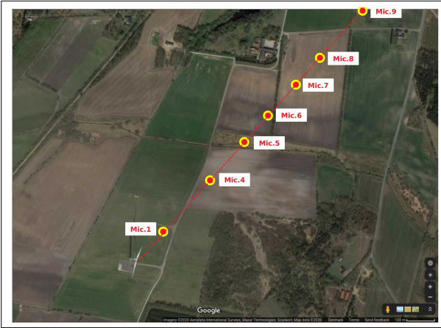
Figure 2. Aerial view of microphone positions along the line (excluding Mic.10 which is positioned further away from the turbine than Mic.9 along the line).
