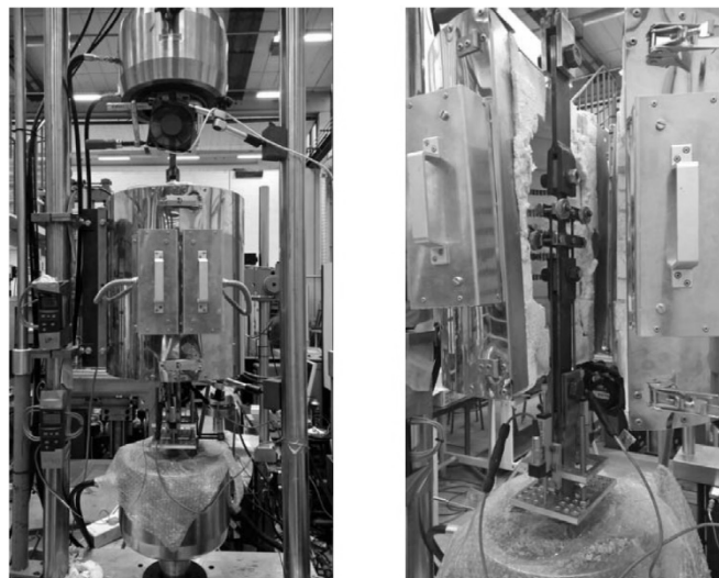
Figure 1: High-temperature monotonic tensile test setup.
