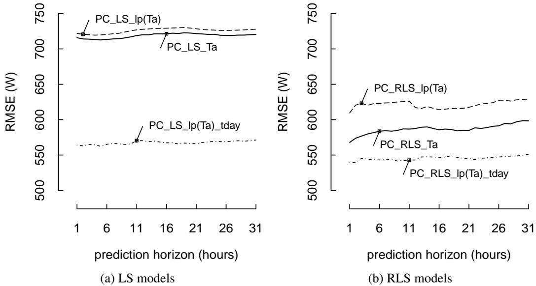
Figure 5.4: Root mean squared error (RMSE) as a function of prediction horizon  $k$ , for the 6 different tested PC-models. A low RMSE indicates better predictions. The same line type is used for the corresponding models in the LS and RLS plot. It is shown that the models including a time of day dependent constant perform best, and that the RLS models outperform the corresponding LS models. Note that the prediction horizon does not affect the RMSE much in these models.
