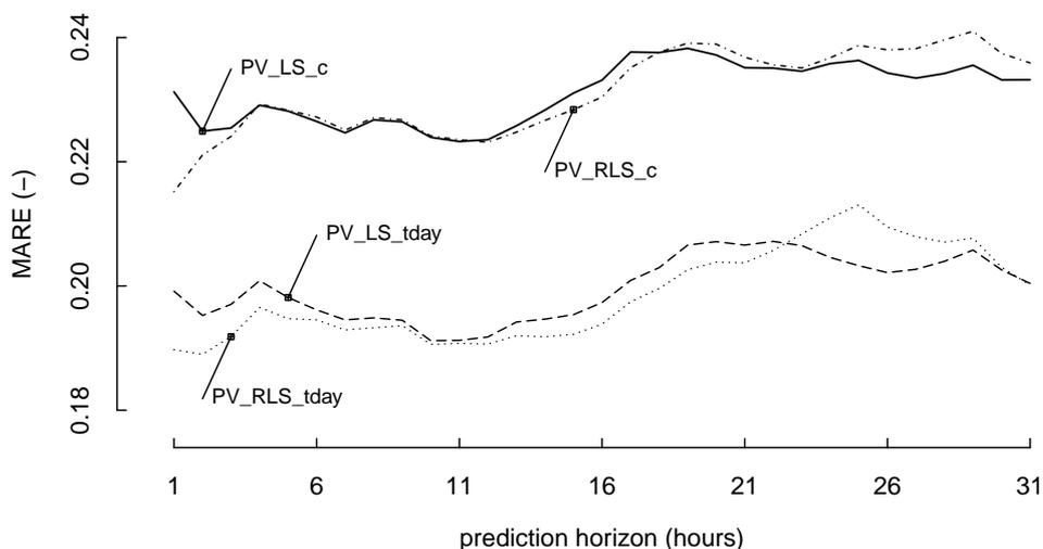
Figure 4.5: Mean Absolute Relative Error (MARE) as a function of prediction horizon  $k$ , for the 4 different tested models. A low MARE is considered better. Again, it is shown that the models including the efficiency as a function of the time of day perform best. In this error measure, the most complex model PV\_RLS\_tday performs best until 22 hours ahead. For larger prediction horizons, model PV\_LS\_tday starts performing better.
