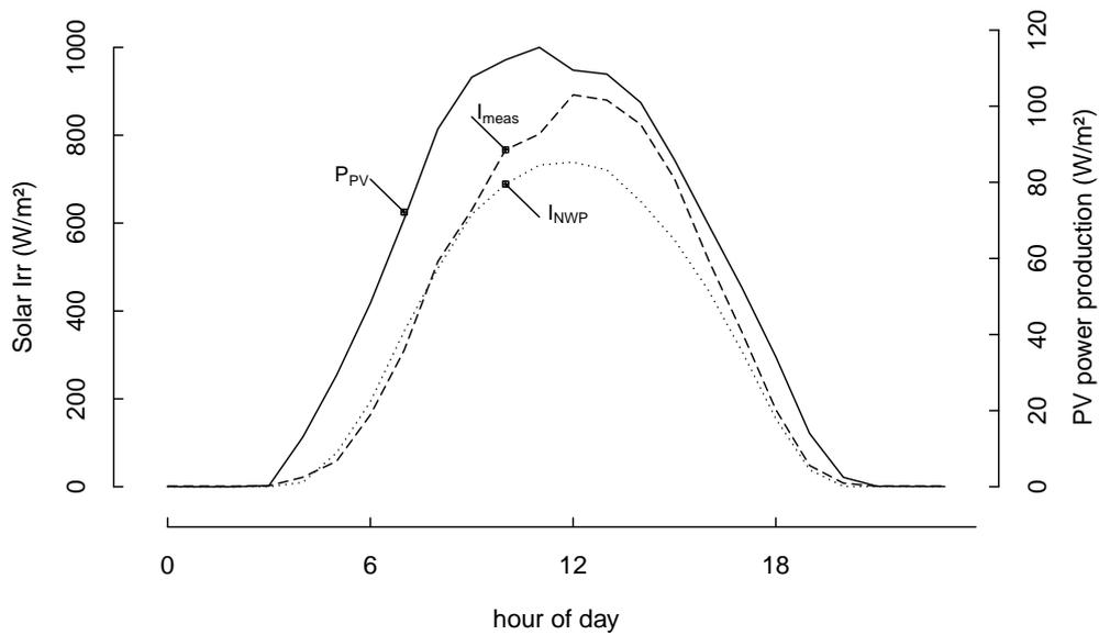
Figure 4.6: The mean of  $P_{pv,t}$ ,  $I_{NWP}$ , and  $I_{meas}$  for each time of day over the test data set. Comparing the solid and dashed line shows that the production is asymmetric with a peak to the left, whereas the NWP of the solar irradiation symmetric. This results in the asymmetry of the estimated efficiency function.
