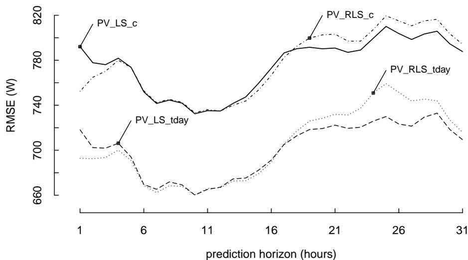
Figure 4.4: Root mean squared error (RMSE) as a function of prediction horizon  $k$ , for the 4 different tested models. A low RMSE is considered better. First of all, it is shown that the models including the efficiency as a function of the time of day perform best. Furthermore, it is visible that the RLS models outperform the corresponding LS models for short horizons from 1-4 hours ahead. After that, the models perform similarly, until the LS model outperforms the RLS for 17-31 hours ahead.
