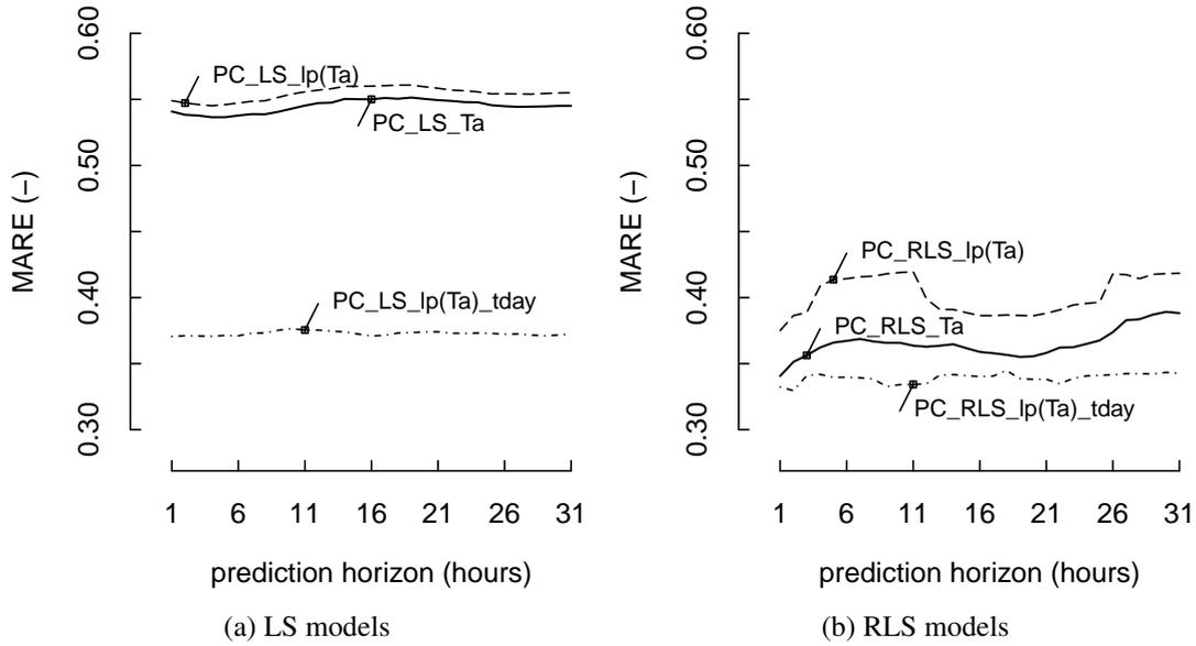
Figure 5.5: Mean Absolute Relative Error (MARE) as a function of prediction horizon  $k$ , for the 6 different tested consumption models. A low MARE indicates better predictions. The same line type is used for the corresponding models in the LS and RLS plot. The hierarchy of model performance is similar to what was observed for the RMSE.
