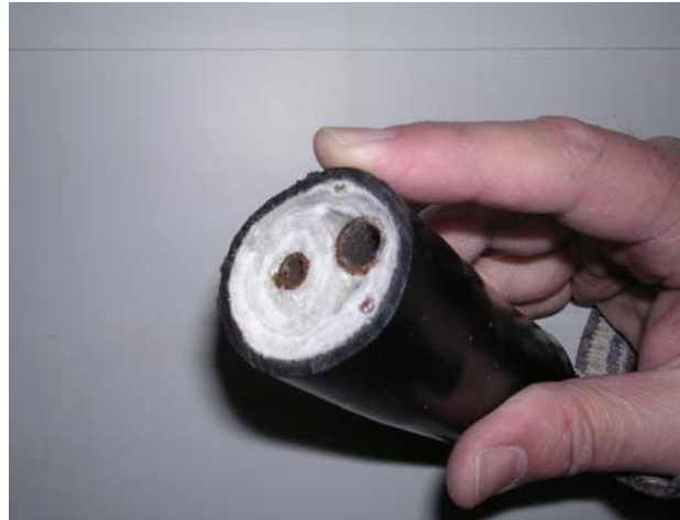
Fig. 2. Lifeline used as solar collector loop in one of the tested SDHW systems.
