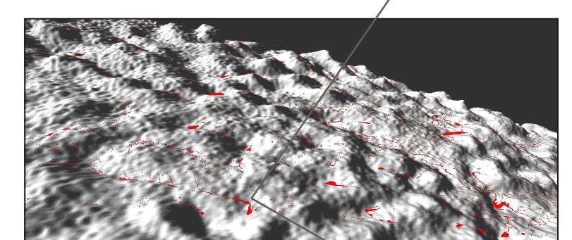
Digital elevation model overlaid by 1999 drainage data (red). The scene is seen from the north and the vertical scale has been multiplied by 50 compared to the horizontal scale.
