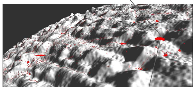
Digital elevation model overlaid by 1999 drainage data (red). The scene is seen from the south and the vertical scale has been multiplied by 50 compared to the horizontal scale.
