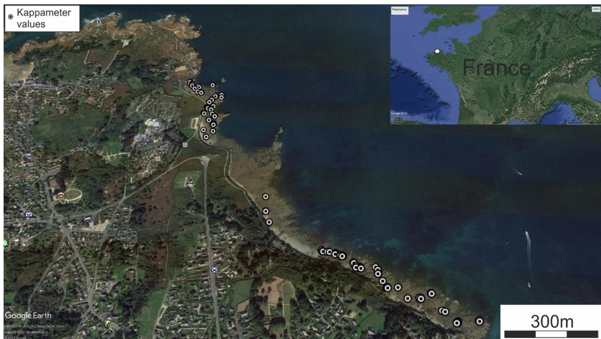
Figure 1 Field area located along and off the coast of Perros-Guirec and Ploumanac in Brittany, France. UAV-borne geophysical mapping was carried out along the entire coast line and about 200m into the water. Black-white dots are locations of kappameter (magnetic susceptibility measurements).
