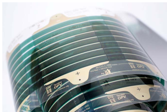
Figure 4. Flexible, ITO-free, vacuum-free OPV module fabricated using continuous roll-to-roll deposition techniques at the Technical University of Denmark.
