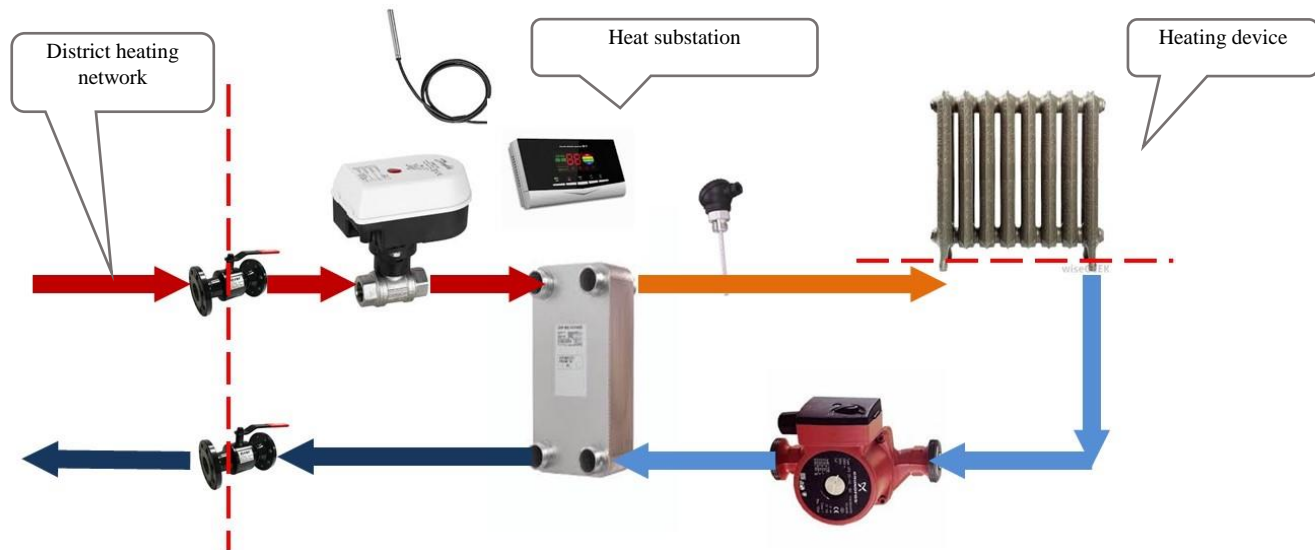
Figure 19. Visualization of energy supply from district heating network to the building level heat substation and energy transition to the heating device
