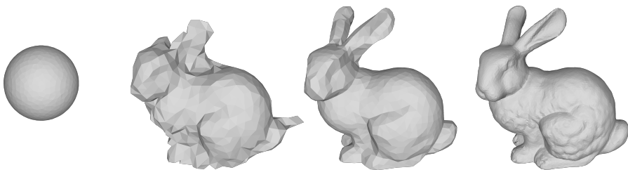
Figure 4.6: The method from Contribution C used to reconstruct the Stanford Bunny starting from a sphere. From left to right: Initial mesh (sphere), after 50 iterations, after 750 iterations, and the converged result. The final reconstruction has 13 780 vertices and a symmetric volume difference error of 0.30%, when compared to the ground truth. Figures is from Contribution C .
