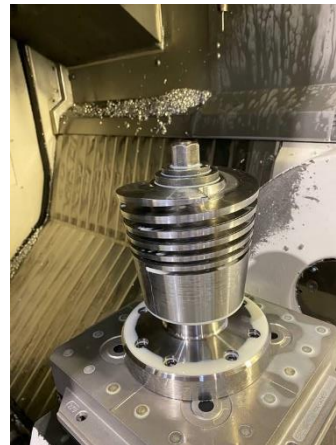
Figure 15: Spindle compressor from Hamburg Vacuum (left) with spindle during production at CSTechcom
