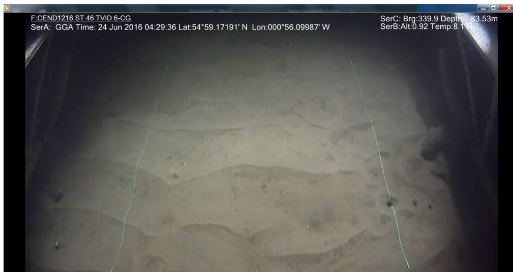
Figure 3.2. Screen grab of video data with field of view defined by stripe laser (81.5 cm).
