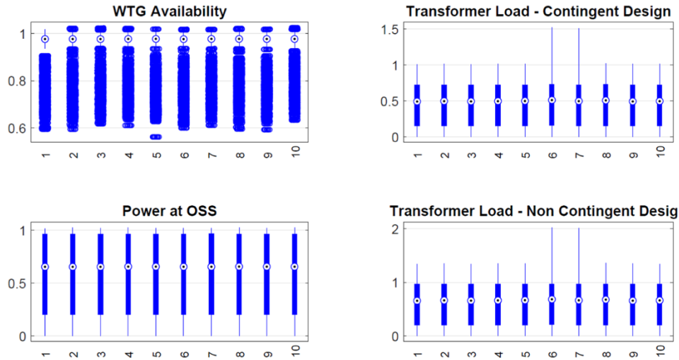
Fig. 12. 10 worst-case scenarios out of 100 scenarios simulated over 15 years showing wind turbine availability, power entering OSS and transformer load for the two design concepts.
