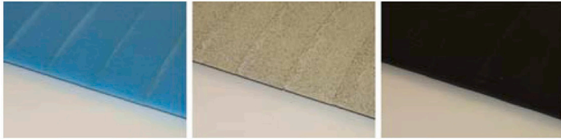
Fig. 31. Some of the porous airfoils used in Geyer et al. [256].
