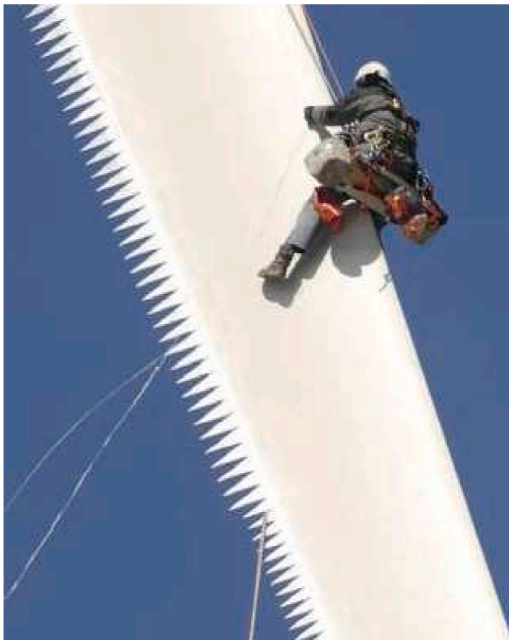
Fig. 36. A typical MW-class wind turbine blade with serrations at the trailing-edge. Source: Oerlemans et al. [223].
