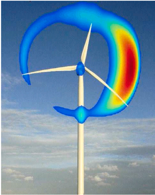
Fig. 35. The noise source distribution in the rotor plane and measured using a microphone array (averaged over many revolutions) is projected on the picture. Source: Oerlemans [284].
