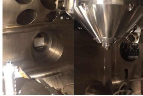
Figure 33: Details of the vacuum chamber showing, on the left, the EBSD detector in its retracted condition. On the right, the bottom of the column where the electron beam is focused to create the desired probe with, on its right, the Everhart-Thornley detector in charge of collecting secondary electrons for imaging purposes. Picture from the author.
