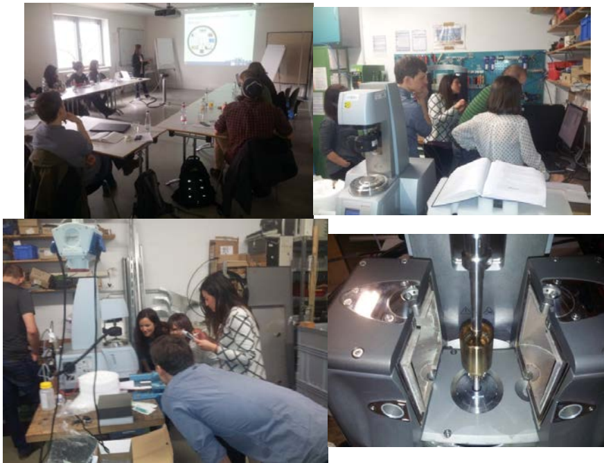
Figure 6: Workshop on measurement of viscosity via rotational rheometers, from above clockwise: Presentations, programming a rheometer, the high temperature measurement geometry filled with molten nitrate salt, filling the gap for the measurement of RT70HC
