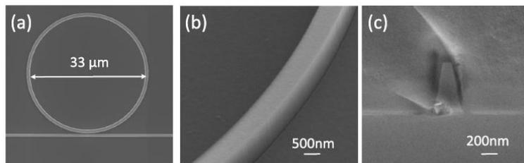
**Figure 2.** (a) Top-view SEM picture of a fabricated SiC microring resonator with 16.5  $\mu\text{m}$  radius. (b) Zoom-in SEM picture of a fabricated microring resonator. (c) Cross-section of an inverse nanotaper at the cleaved facet [2].
