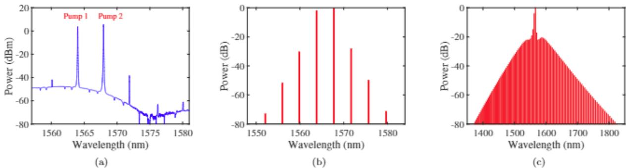
**Figure 3.** (a) The measured spectrum of the TE polarized dual-pump OPO in a 4H-SiC microring resonator. The adjacent frequency lines are separated by one FSR. (b) The simulated result of the TE polarized dual-pump OPO in a 4H-SiC microring resonator. (c) The simulated result of soliton frequency comb generation through thermal tuning [3].
