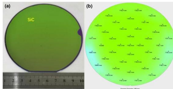
**Figure 1.** (a) Photograph of 4-inch wafer-scale 4H-SiCOI substrate fabricated using ion-cutting and layer transferring technique. (b) The thickness homogeneity of SiC film was measured by white light interferometer [1].
