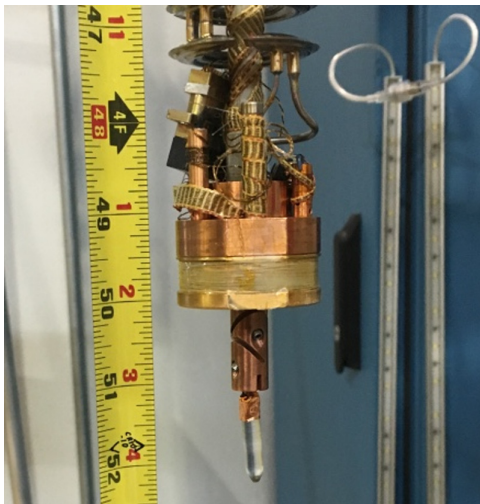
FIG. 15. Crystal used for neutron scattering experiments and susceptibility measurements.
