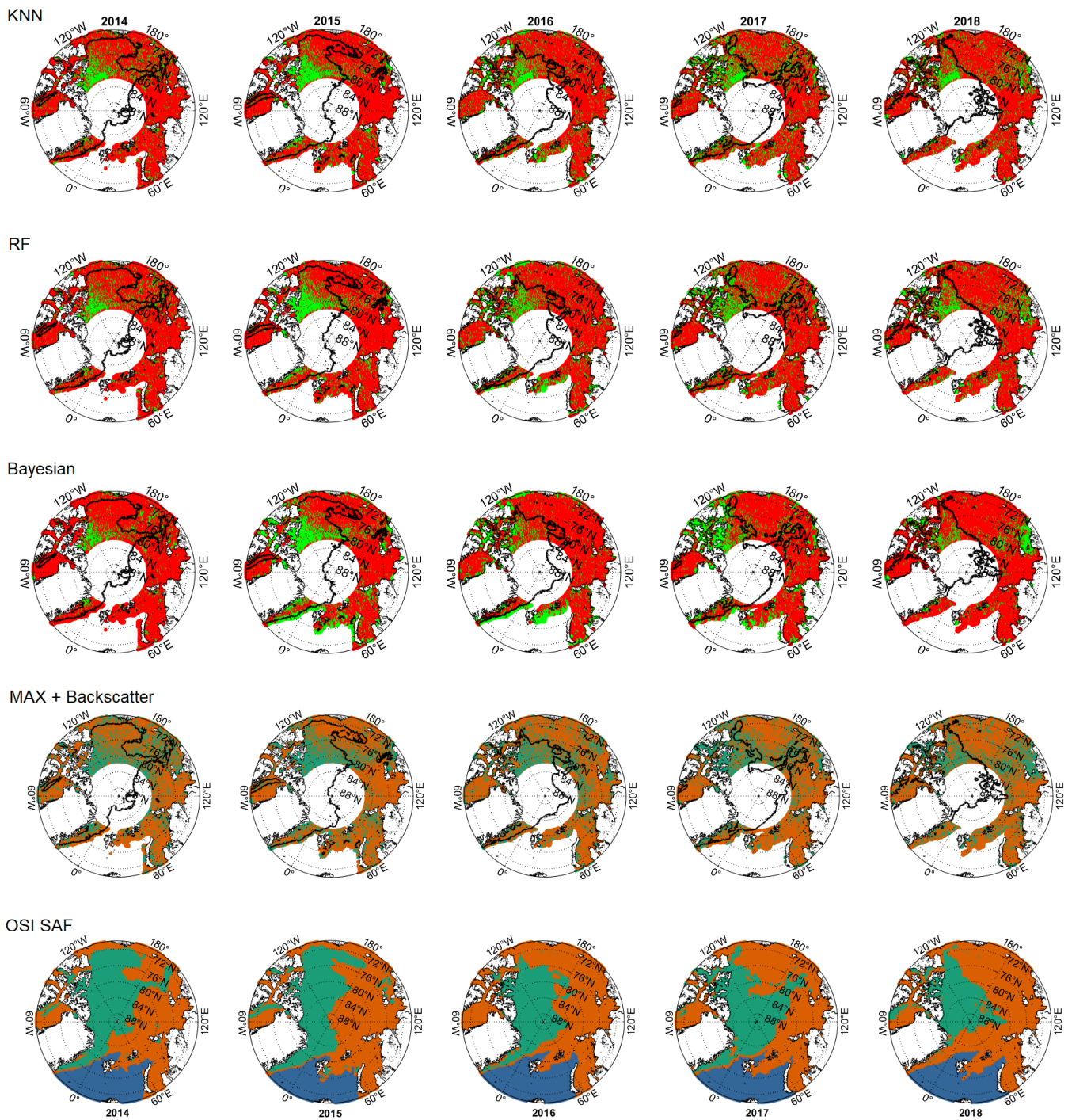
Figure 7. Classification of sea ice types by AltiKa radar echo waveforms in February (35 day cycle) 2014–2018, with KNN, RF and Bayesian classifiers (supervised classifiers), using a combination of waveform parameters LEW + \sigma_0 and a threshold-based classifier using waveform parameters MAX + \sigma_0 . For the supervised classifiers, FYI is denoted by bright red and MYI by bright green. For the threshold-based classifier, FYI is denoted by brown and MYI by green. For reference, OSI SAF sea ice type is presented with FYI denoted by brown, MYI by green and open ocean by blue. Black contour lines denote the MYI/FYI edge provided by OSI SAF.
