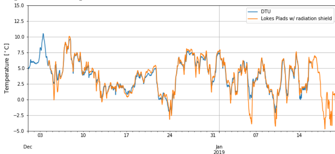
Figure 2-2 Comparison between outdoor temperature measurements in Stengården and DTU Kgs. Lyngby.
