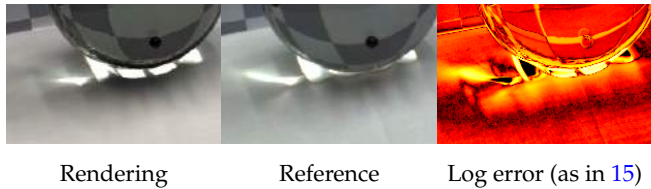
Fig. 21. Effect of separating markers from glass (refracted light close to marker) and of not accounting for subsurface scattering (dark areas close to caustics).
