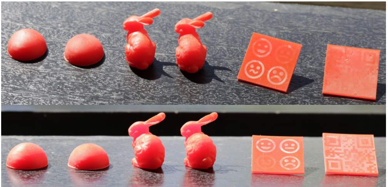
Figure 1: Hemispheres and bunnies with smooth and rough surfaces, and flat samples (smileys and QR code) with spatially varying anisotropic reflectance. The scene is observed from two different directions to exhibit the anisotropy. The sun is used as a directional light source. Each item was printed in a one-step process using the presented technique.
