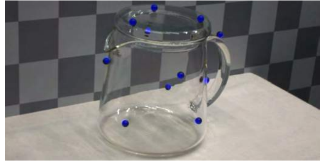
Fig. 14. Markers rendered in blue and added to the reference image to validate marker positions by looking at pixel offsets.
