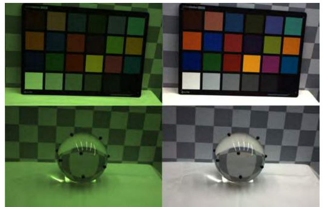
Fig. 10. Color calibration: raw images (left) and color corrected images (right). The camera sensor is particularly sensitive to green.
