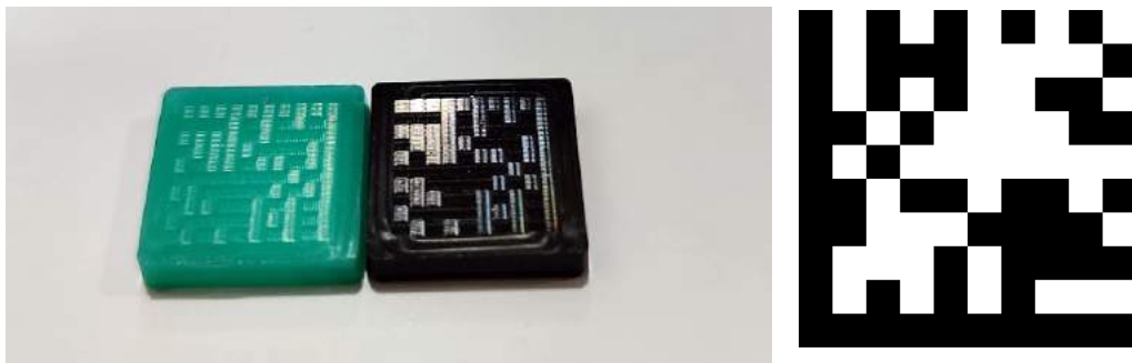
Figure 4.2: Left: Image showing two datamatrix samples used in Contribution C . They are made from injection molding with the micromilled ridged structures. Both specimens are translucent, but the green sample is see through, where the black sample has a higher absorption. This strongly influences the contrast, as can also be seen in the image. Right: Datamatrix code for "DTU".
