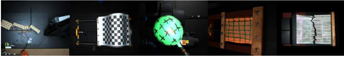
Figure 4.11: Images of the 5 different small robots made for the dataset in Contribution F . Each representing a different type of non-rigid deformation. Starting from left to right, Articulated, Bending, Deflation, Stretching, and Tearing.
