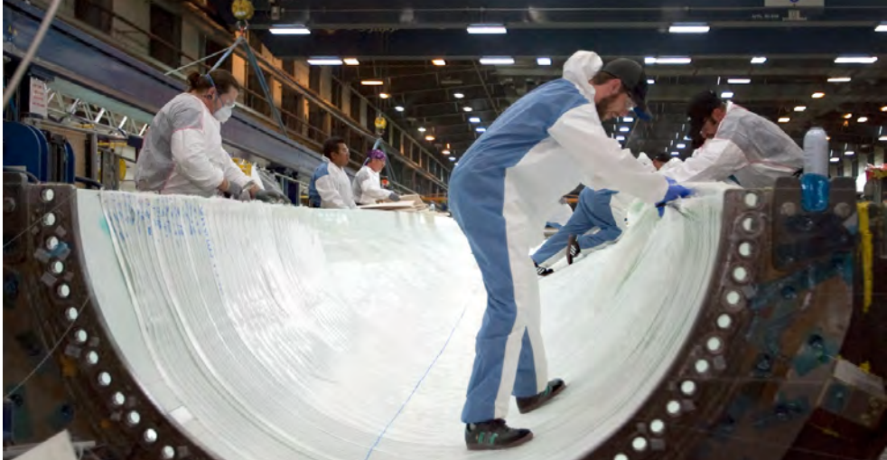
Figure 2.2 – Blade technicians at Vestas Wind Systems manufacturing plant in Windsor lay fiber material in a shell of a wind turbine blade. Photo by BizWest/Joel Blocker, 2015. Published by BizWest, June 30 2017.
