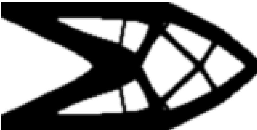
(b) A filter radius of 1.5 is applied on the densities, which resolves the problem of checkerboard elements. Note how the border between solid and void regions becomes grayscale due to the regularization.
