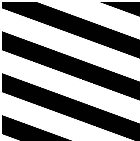
Figure 2.2: Two-phase composite with solid and void phase. This composite is also called rank-1 material.
