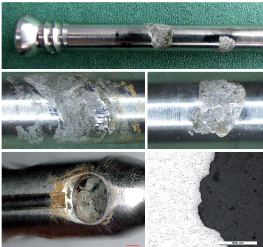
Figure 10. Mechanically assisted crevice corrosion/fretting and crevice corrosion at a locking screw, screw hole including microscopic image of the corrosion-attacked microstructure. For SEM imaging see Figures 12 and 13 in Supplementary data.
