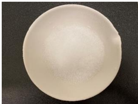
Figure 3.3 Methane hydrate powder, ranging from 250 to 400 microns.
