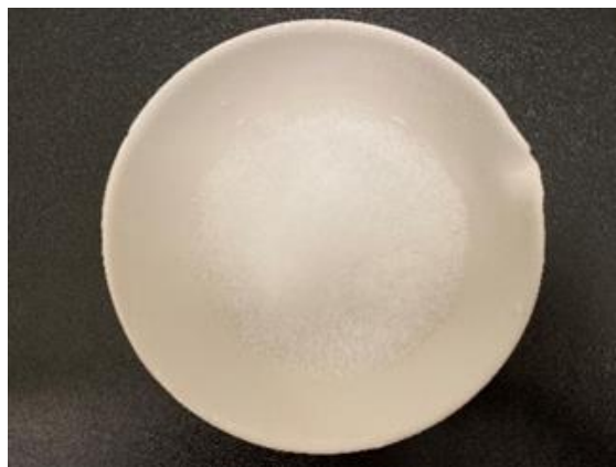
Figure 3.3 Methane hydrate powder, ranging from 250 to 400 microns.
