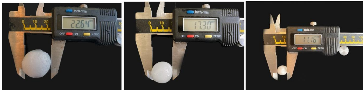
Figure 3.4 Spheritic hydrate samples were synthesized at diameters of 22 mm, 18 mm, and 11 mm.
