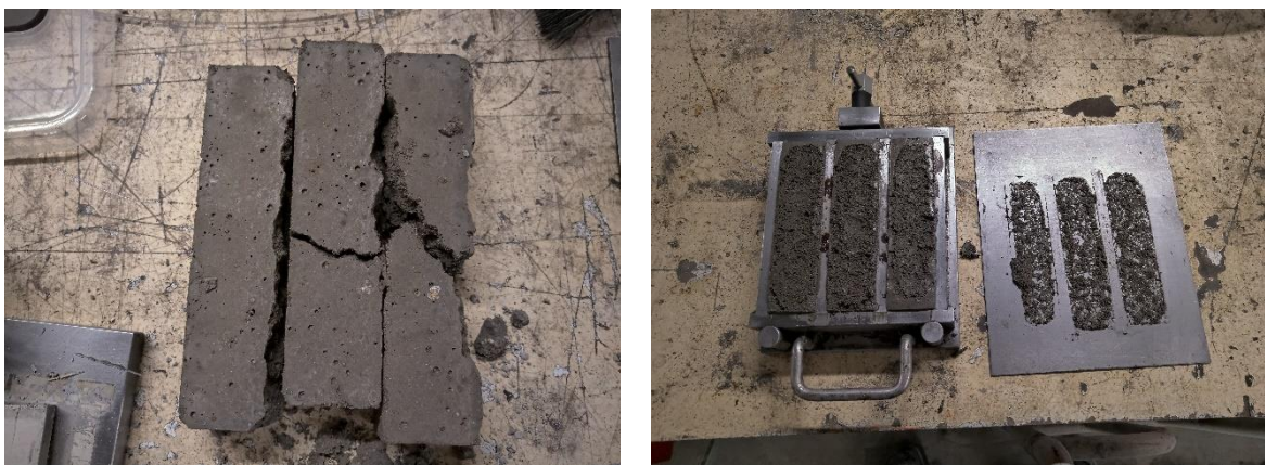
Figure 27: Demoulding of mortar with AMA (left) and NUU (right) after 24 hours.
