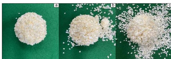
Fig. 4. Rating for the clump breakage: (a) clump intact (no breakage), (b) slightly broken and (c) moderately broken.
