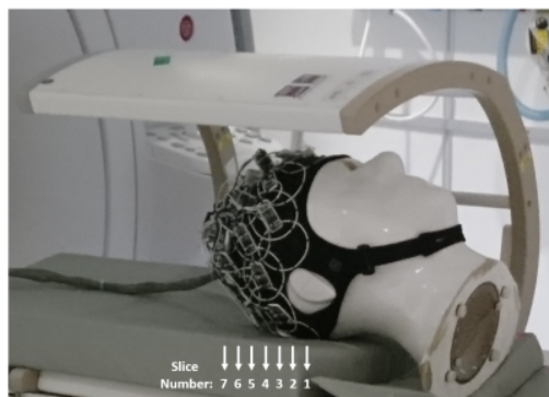
Figure 2. Fabricated flexible 32-channel ^{13}\text{C} receive-only array ( f = 32.1 MHz), attached to the head phantom used for MR characterization. The projection of the 7 slices used for the volumetric characterization is also noted.
