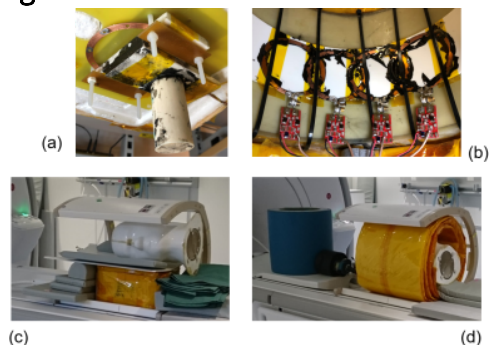
Fig. 1. Experiment setups. (a) Setup 1. The cylindrical ceramic part stands in liquid nitrogen (LN 2 ) and cools the coil to -169°C (104 K). (b) Setup 2 for the 4-channel array. The fiberglass LN 2 chamber underneath is connected to a LN 2 tank, and the inner and outer surfaces are clad in Aerogel layers, as shown in (d). The temperature goes to -162°C (111 K). Coil-to-sample distances are around 22 mm for (a) and 13 mm for (b). (c) Setup 1 and (d) setup 2 at an MR scanner.
