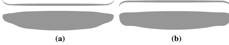
Fig. 12 Elevation and plan views of unswept optimized designs for (a) raised and (b) drooped wings.
