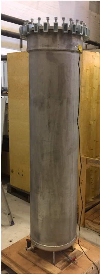
Fig. 1. The heat storage unit without insulation.
