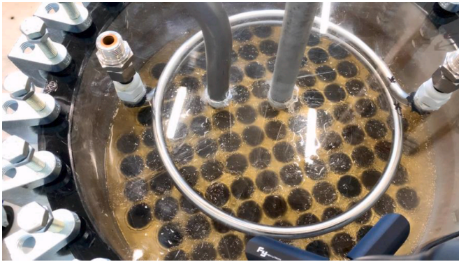
Fig. 2. The manifold plate with a view of the tubes inside the storage (PCM was melted).
