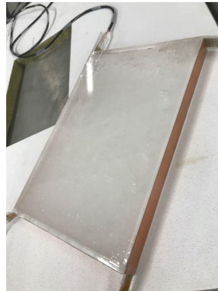
Figure 4-2: PMMA sample containing PCM with the lateral heat flux meters before installation in the insulation
