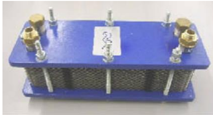
FIGURE 5-3: COMMERCIALY AVAILABLE PLATE AND FRAME HX EVALUATED BY MEDRANO ET AL. (2009).
