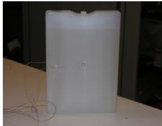
FIGURE 5-22: MACROENCAPSULATION OF ORGANIC PCM DERIVED FROM RENEWABLE AND BIO-BASED; CRODATHERM™ 53 ; T_{MELTING}: 53^{\circ}\text{C}
