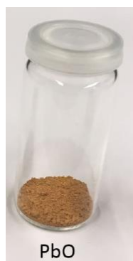
FIG. 5A: RAW MATERIAL (PbO); FIG. 5B: ISOTHERMAL STORAGE CYCLE AT 500 °C BETWEEN PbCO 3 ·2PbO AND PbO TRIGGERED BY A CHANGE IN CO 2 PRESSURE FROM 8 TO 2 BAR
