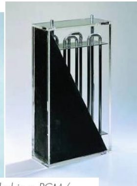
Shell-and-tube heat exchanger embedded in a PCM/graphite heat storage compound (SIGRA \lambda )
