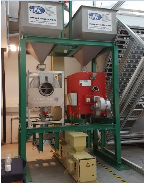
FIGURE 3-23 ROTATING BED OPEN HEAT STORAGE PROTOTYPE DEVELOPED IN PROJECT OFFSOR.
