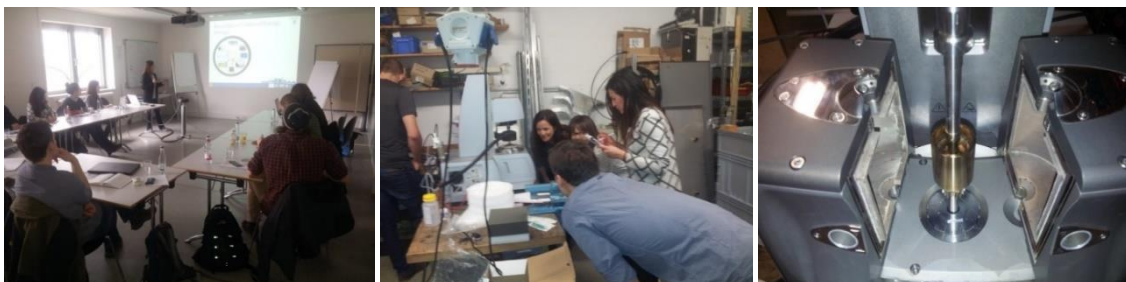
FIGURE 1.2-7: WORKSHOP ON MEASUREMENT OF VISCOSITY VIA ROTATIONAL RHEOMETERS, FROM LEFT TO RIGHT: PRESENTATIONS, THE HIGH TEMPERATURE MEASUREMENT GEOMETRY FILLED WITH MOLTEN NITRATE SALT, FILLING THE GAP FOR THE MEASUREMENT OF RT70HC
