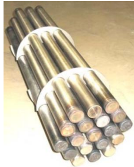
FIGURE 5-11: BUNDLE OF CYLINDERS CONTAINING PCM FOR HIGH TEMPERATURE APPLICATIONS (SOURCE: BUSCHLE ET AL. 2006).
