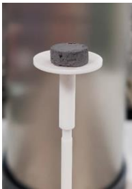
FIGURE 3. CILINDRIC POROUS PELLETS USED FOR TG ANALYSIS.
