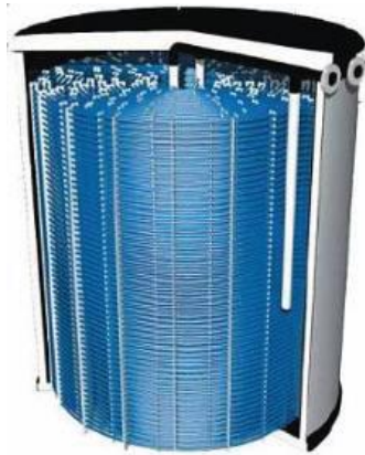
CROSS SECTION OF CALMAC'S ICEBANK® COLD STORAGE SYSTEM (SOURCE: CALMAC, MEHLING AND CABEZA 2008)
