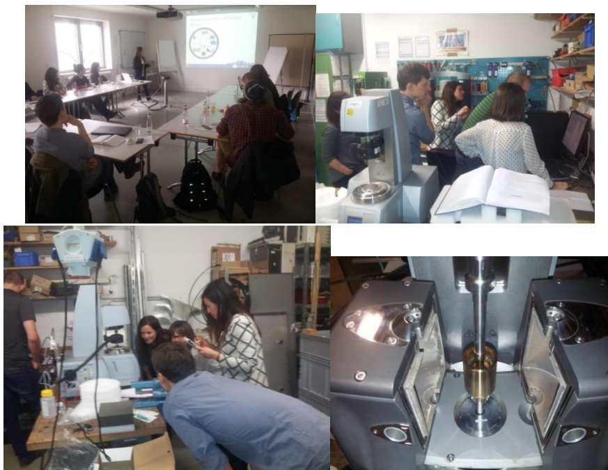
FIGURE 3-8: WORKSHOP ON MEASUREMENT OF VISCOSITY VIA ROTATIONAL RHEOMETERS, FROM ABOVE CLOCKWISE: PRESENTATIONS, PROGRAMMING A RHEOMETER, THE HIGH TEMPERATURE MEASUREMENT GEOMETRY FILLED WITH MOLTEN NITRATE SALT, FILLING THE GAP FOR THE MEASUREMENT OF RT70HC
