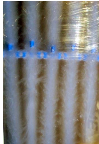
PCM CRYSTALLIZING AT CAPILLARY TUBES (SOURCE: ZAE BAYERN)
