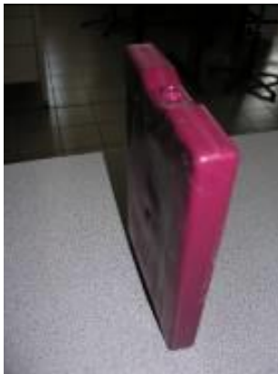
FIGURE 5-21: MACROENCAPSULATION OF HYDRATED SALTS IN POLYOLEFIN BRICK; CRISTOPIA T_{MELTING}: 27^{\circ}\text{C}
