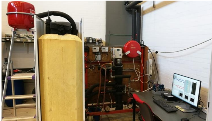
FIG.: PCM HEAT STORAGE TEST FACILITY AT DTU BYG (LEFT); SCHEMATIC OF CHARGE AND DISCHARGE LOOP (RIGHT).
