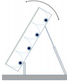
Fig. 1: The diagram of cross-section of PolyCSP CPC collector
