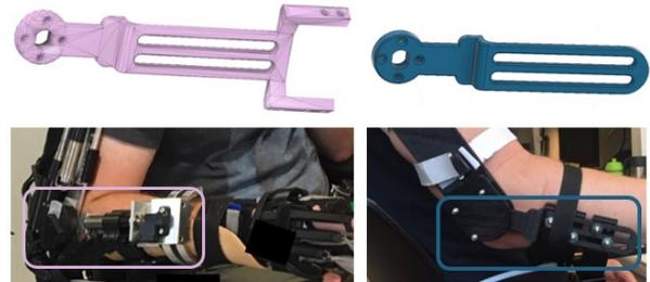
Fig. 4: The elbow connection of the existing EXOTIC exoskeleton and the new design. The existing design was shaped as a fork (pink) to carry the motor and C-shaped wrist rail. The new design (blue) was shorter, as it only carried the elbow rest and the passive joint.
