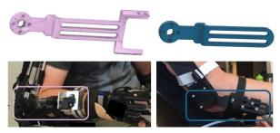
Fig. 4: The elbow connection of the existing EXOTIC exoskeleton and the new design. The existing design was shaped as a fork (pink) to carry the motor and C-shaped wrist rail. The new design (blue) was shorter, as it only carried the elbow rest and the passive joint.
