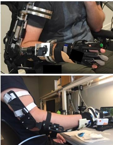
Fig. 2: Comparison: *top*) The existing EXOTIC exoskeleton, *bottom*) The new design proposed in this study.
