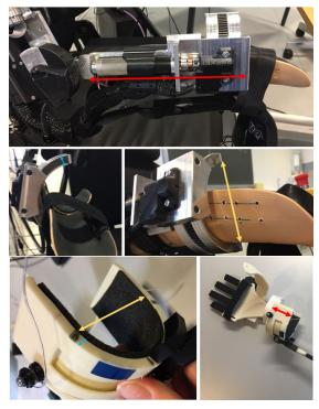
Fig. 10: The measured entities referenced in Table II, red is the length, blue is the width, and yellow is the diameter of the C-shape and U-shape, respectively. The top three images show the EXOTIC design, and the bottom two images show the new design.
