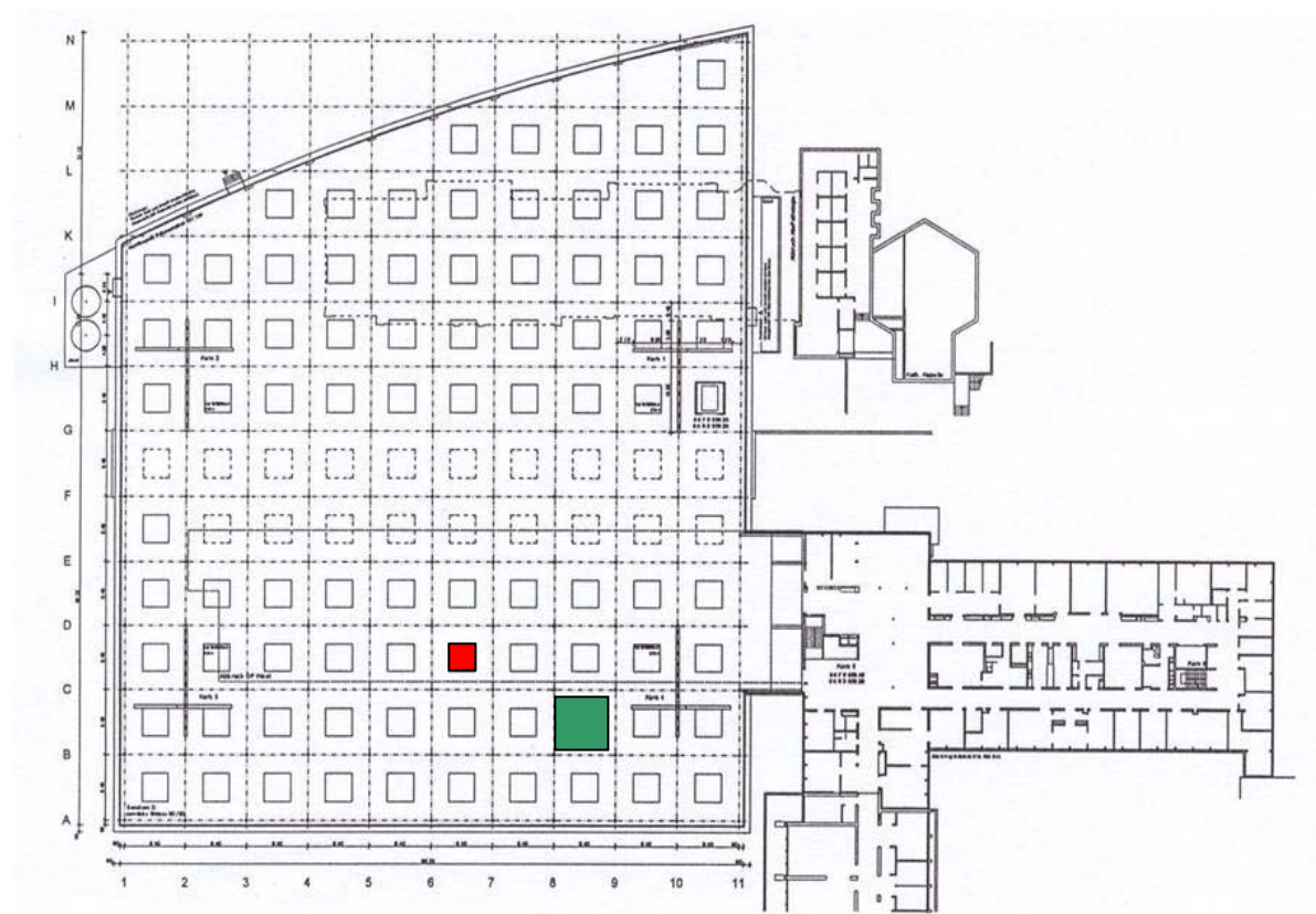
Figure 3: Plan of a typical floor of the Primary System, showing 8.4m x 8.4m structural grid. The primary System architect was Peter Kamm and Kundig, Architects. This firm
