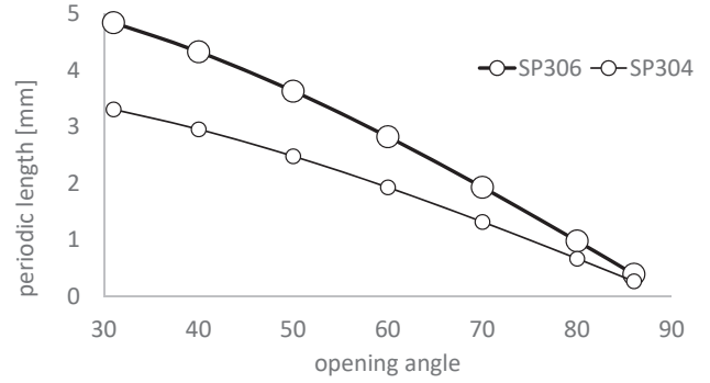
Figure 11 Periodic spacing \Delta_{SP} versus opening angle \varphi
