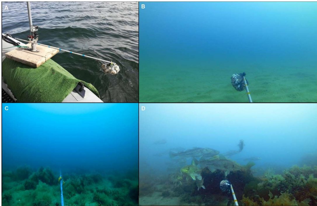
Figure 4.2 – Multi-pane overview of the RUUVS used for monitoring in this study. A) BRUVS setup with a bait arm extended within the FOV, marked with tape at 10 cm increments used for visibility estimates, B) Sand site with low cobble coverage recorded by a BRUVS, C) Reef site with high cobble coverage, recorded by an UBRUVS with a sponge attached to a rope at 1 m distance from the camera for visibility estimates and D) a school of Atlantic cod ( Gadus morhua ) passing the FOV, recorded at intermediate cobble coverage by a BRUVS at one of the reef sites.
